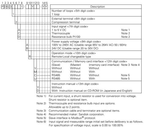
For specification of thermocouple, K, 0.0 to 400.0°C.
