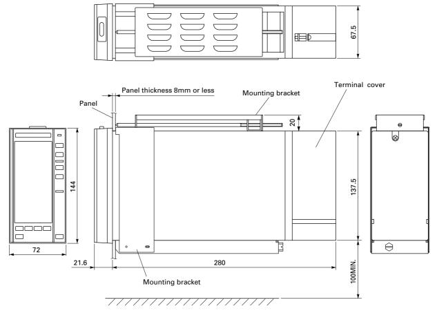
Note) The distance between other instruments and low end of PDG shall be more than 100mm.
